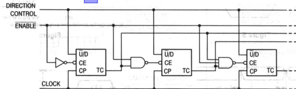
Figure c. Synchronous n-Stage Counter with Parallel Gated Carry/Borrow
