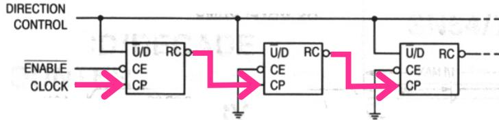
Figure a. n-Stage Counter Using Ripple Clock
