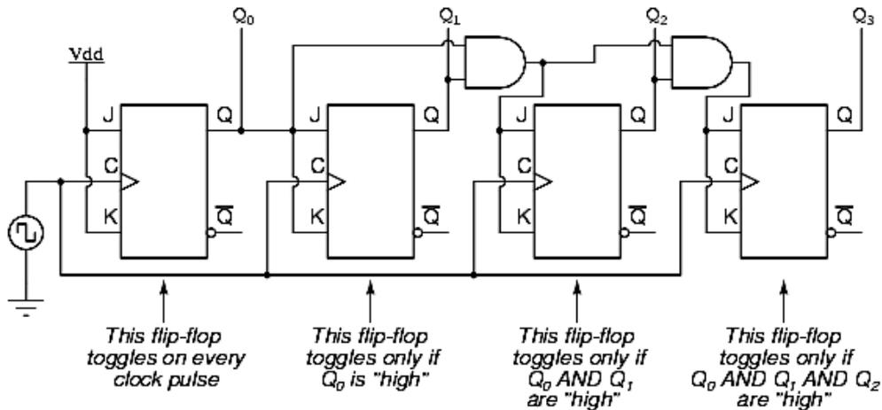
*A four-bit synchronous "down" counter*
