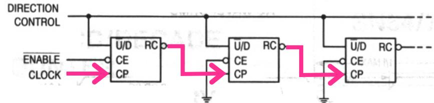
Figure a. n-Stage Counter Using Ripple Clock
