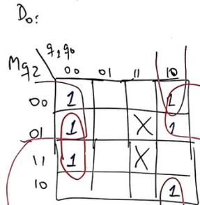
$$D_0 = \bar{M} \cdot \bar{q}_0 + \bar{q}_2 \cdot q_1 \cdot \bar{q}_0 + q_2 \cdot \bar{q}_1 \cdot \bar{q}_0$$
