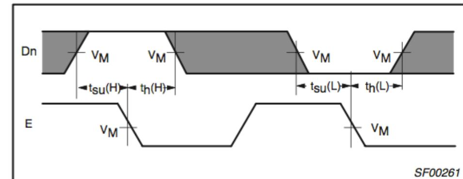
Waveform 4. Data set-up time and hold times
