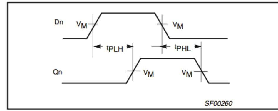
Waveform 3. Propagation delay for data to output
