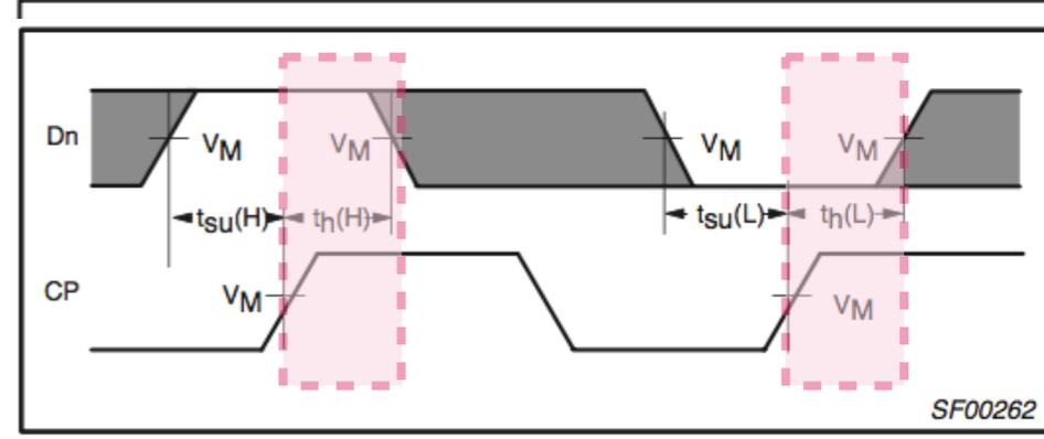
Waveform 5. Data set-up time and hold times
