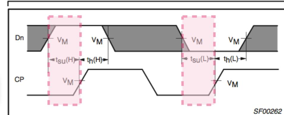
Waveform 5. Data set-up time and hold times
