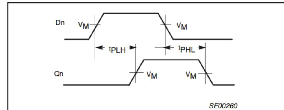
Waveform 3. Propagation delay for data to output
