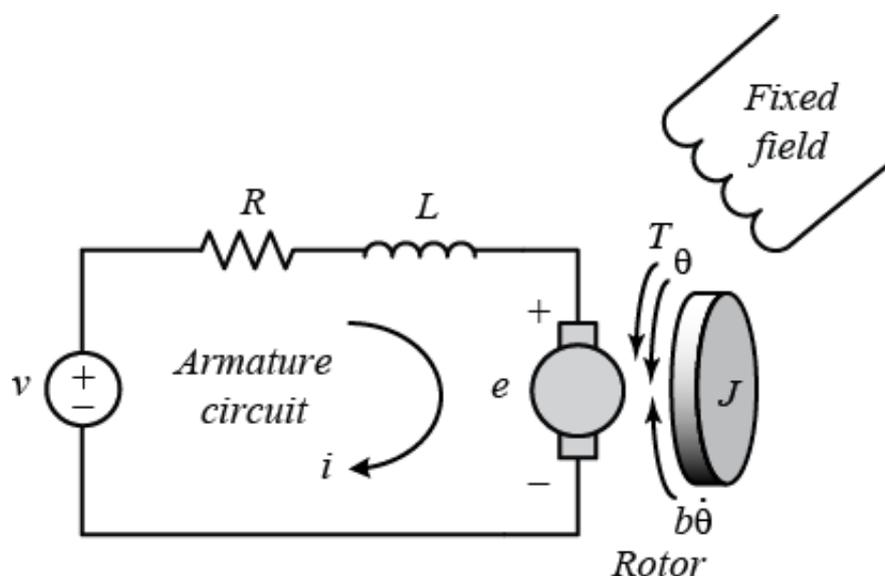
For this example, we will assume that the input of the system is the voltage source ( $v$ ) applied to the motor's armature, while the output is the rotational speed of the shaft  $\dot{\theta}$ . The rotor and shaft are assumed to be rigid. We further assume a viscous friction model, that is, the friction torque is proportional to shaft angular velocity.
