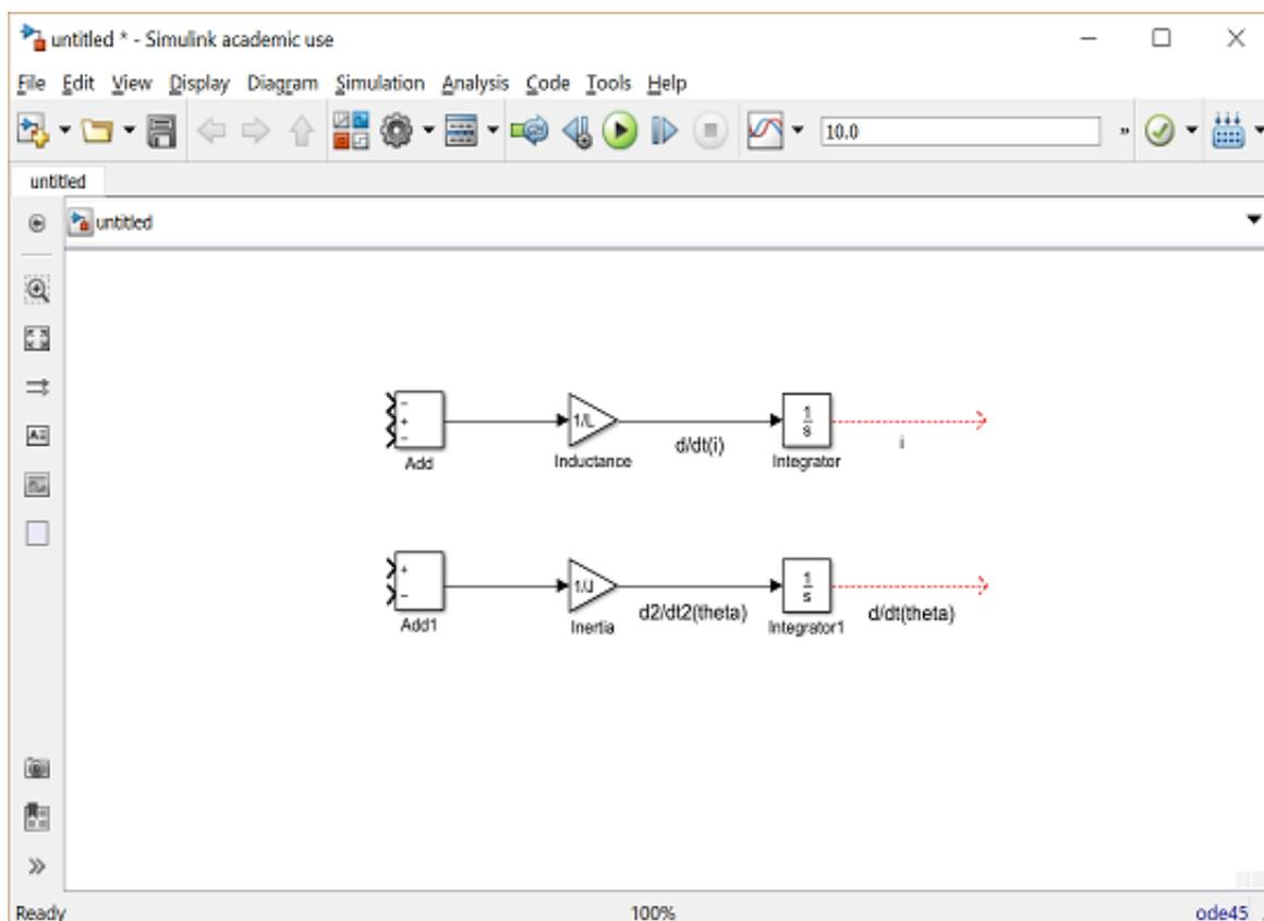
Now, we will add in the torques which are represented in the rotational equation. First, we will add in the damping torque.
